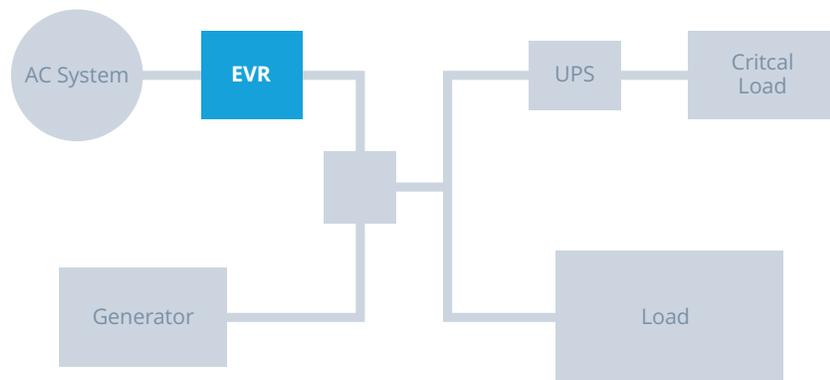
**Option B** supplements Option A with an EVR, which allows the system to remain at full power without diesel backup during power surges, sags and brownouts of any duration. The addition of the EVR not only reduces reliance on diesel, but it also reduces wear and tear on the UPS. Because the EVR will compensate for all surges, sags and brownouts, the UPS will have fewer on/off cycles and less required maintenance.
