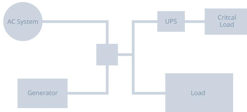
**Option A** depicts a system that has, for the past quarter century, been applied to mitigate power anomalies. Option A relies upon a UPS to provide sag and surge protection and to supply full power to sensitive and critical loads (~15%) during brownouts. It also relies upon diesel generation to power essential services, such as HVAC, refrigeration and elevators.
